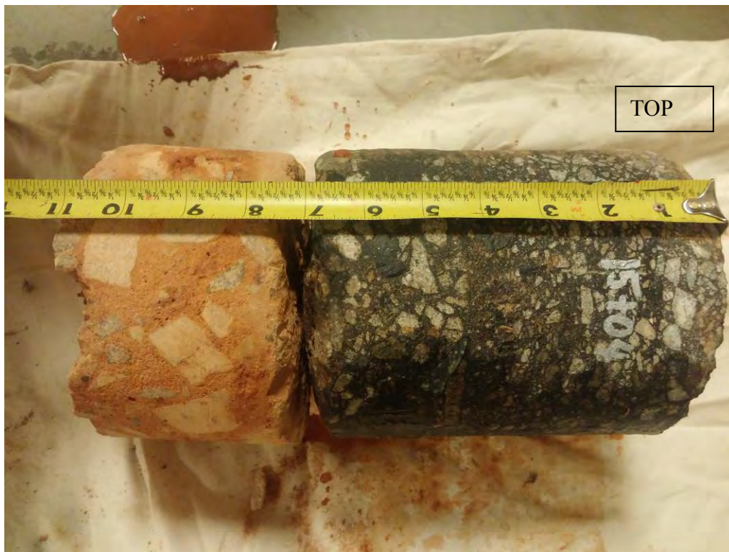
CORE 2 – GREEN STREET – STATION 15 + 04±, SB, LANE 1, 5' RT OF CL
