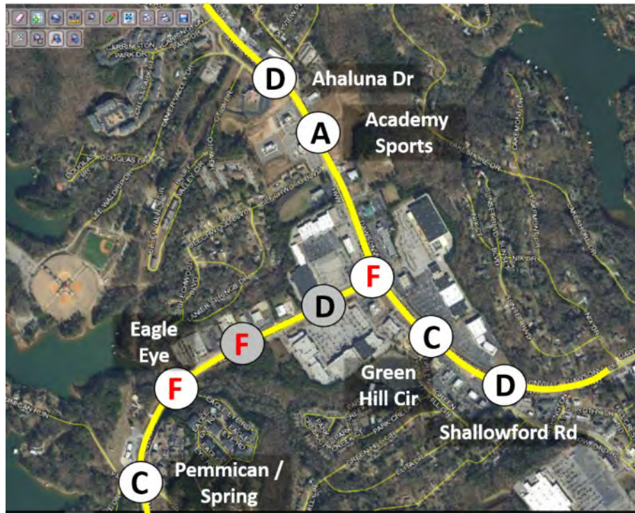
FIGURE 17. 2040 NO-BUILD LEVEL-OF-SERVICE - PM PEAK
