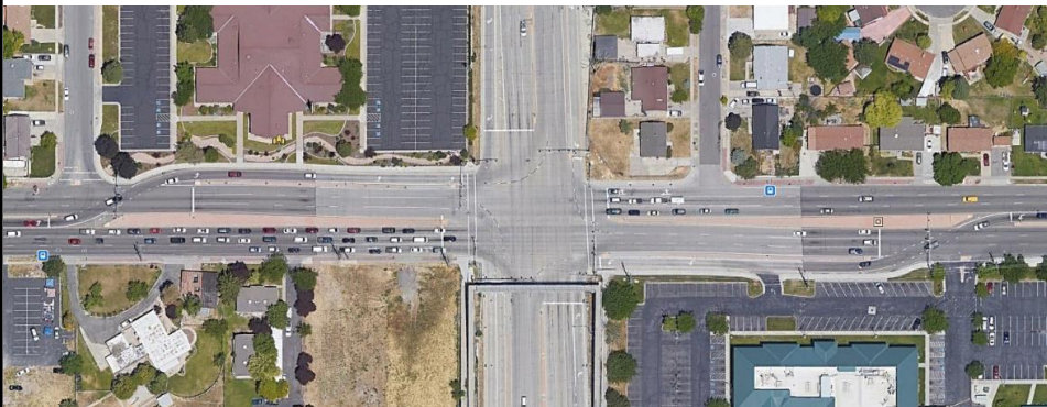
CFI located in Salt Lake City, UT
